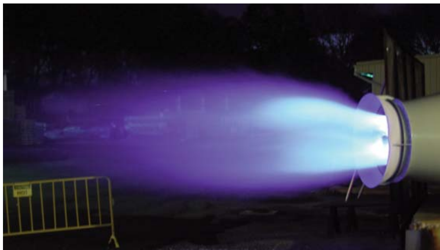
NovaStar NS150 firing natural gas at 140 MMBtu/hr
